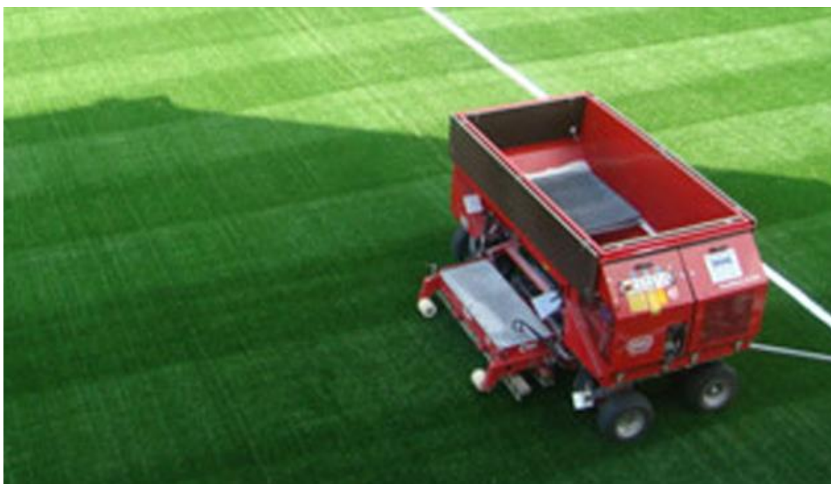
Figure A 8: Mechanised application of infill (photo submitted by ESTO)
