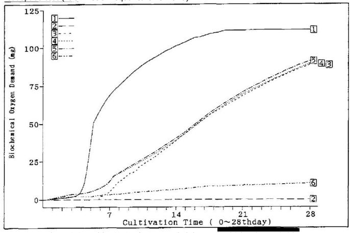
MITI I Test according to OECD guideline 301C: reference control, sludge + aniline (1) / sterile controle (2), water + test substance / test vessel (3) (4) (5) / control blank (6)
