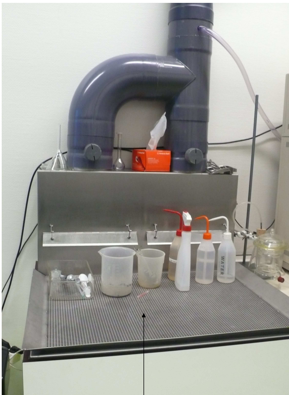
The suction below the working area
