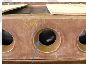
Cathode/Diaphragm covered with black sheets
