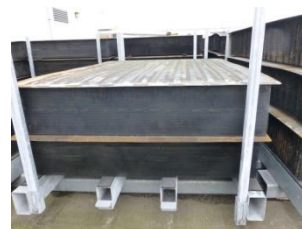
Anodes for reuse
