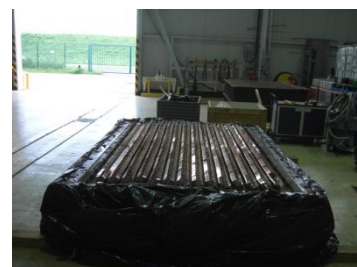
Removed sheets from cathode
