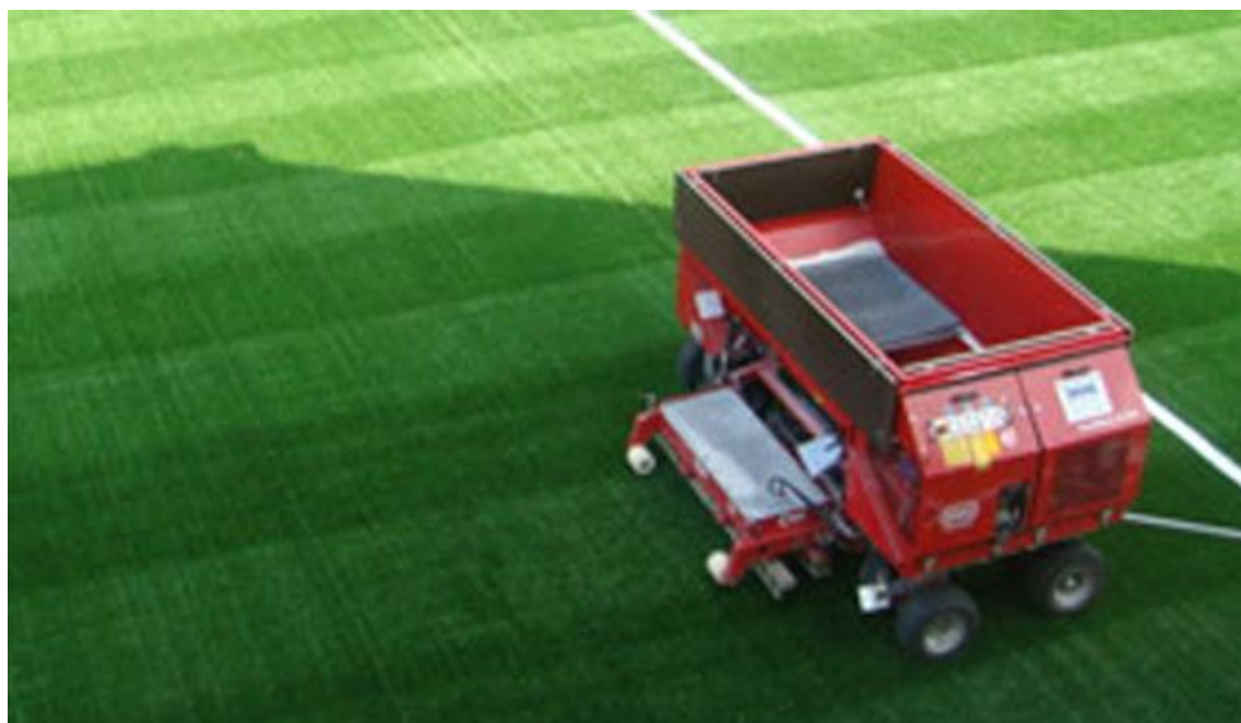
Figure 2: Larger operators with automated infilling system
