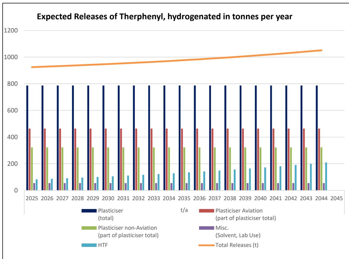
The worst-case cumulative releases of Terphenyl, hydrogenated from 2025 to 2044 have been estimated with a total volume of 19 584 tonnes, which corresponds to an average annual release of 979 tonnes. From 2025 to 2044 the annual releases increase from 925 to 1 052 tonnes, as illustrated in **Table 18**.
