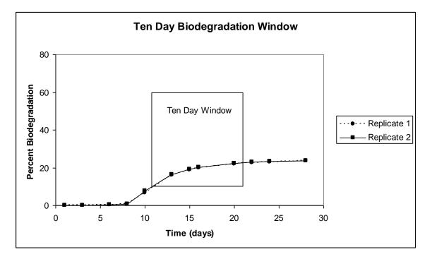
Figure A7.1.1.2.1/02-2: Ten Day Window for the Biodegradation of <sup>14</sup>C-BIT
