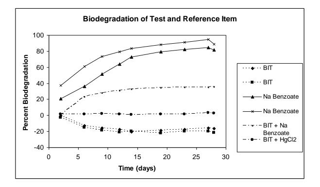
Figure A7.1.1.2.1-1: Biodegradation of the test item and the reference item during incubation period
