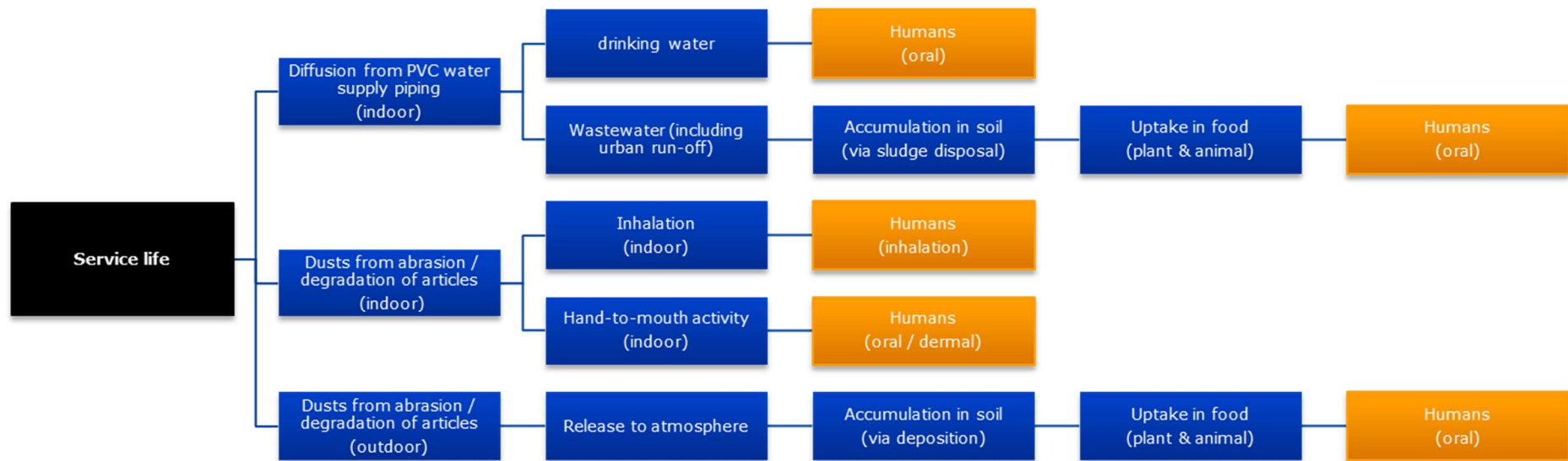
Figure 1. Conceptual exposure pathways for humans relevant to the service life of PVC articles
