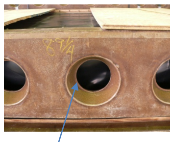
Cathode/Diaphragm covered with black sheets
