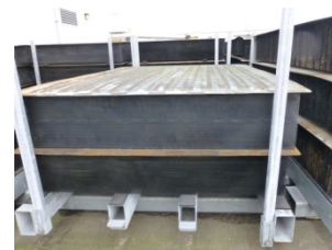
Anodes for reuse
