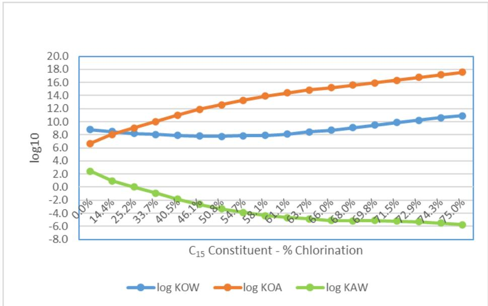
Figure 5: Plots of  $K_{OA}$ ,  $K_{OW}$  and  $K_{AW}$  for CPs - C<sub>15</sub> constituents (Endo, 2021)
