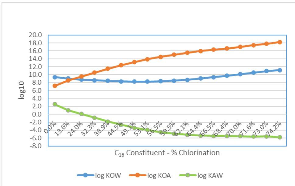
Figure 6: Plots of  $K_{OA}$ ,  $K_{OW}$  and  $K_{AW}$  for CPs - C<sub>16</sub> constituents (Endo, 2021)
