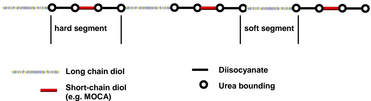
Figure 4: Polyurethane chain with hard segments with MOCA as short-chain diol and soft segments with long-chain diols. (Adapted from Gregori et al. 2007)
