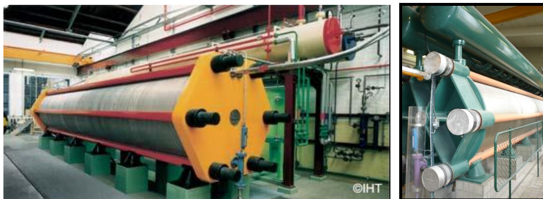
Four cellblocks mounted together, IHT construction on the left and AAK on the right
